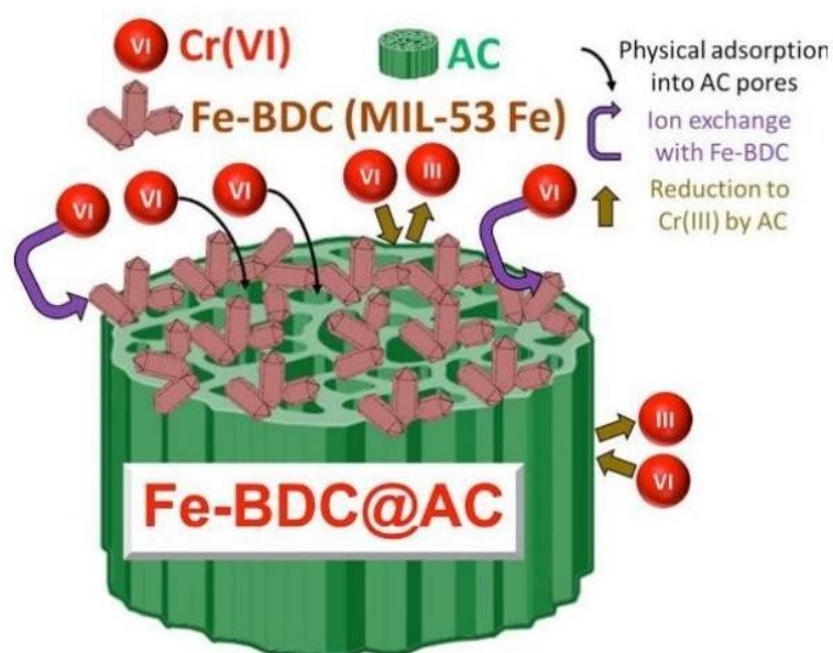
Fig. 16 of proposed adsorption mechanism of Cr (VI) onto Fe-BDC@AC [10]
