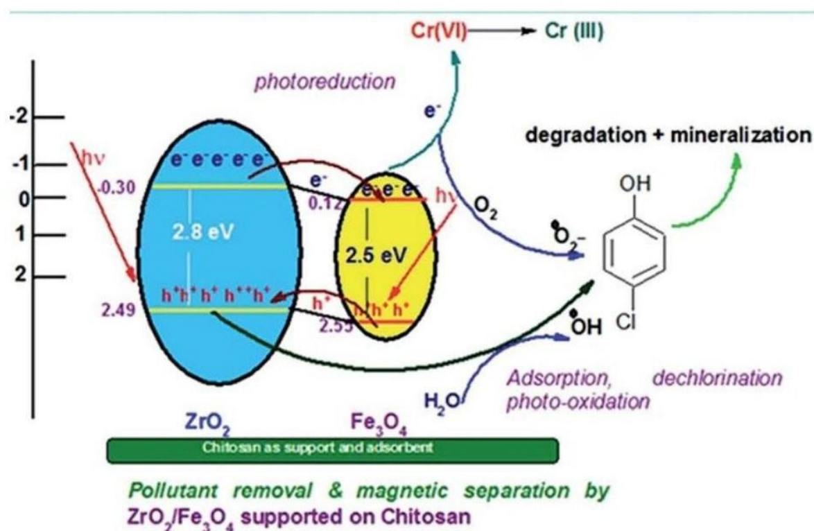
Fig.27 Removal of Cr (VI) using chitosan [20]
