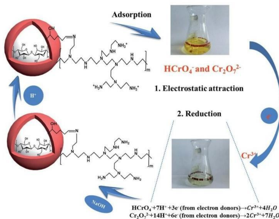
Scheme 2 The mechanism for the removal of Cr(vi) by CPA-2.
