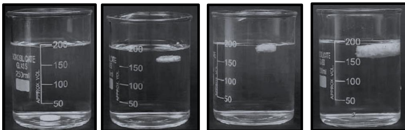
Figure 7.8 Buoyancy/floating study of Lovastatin tablet.
