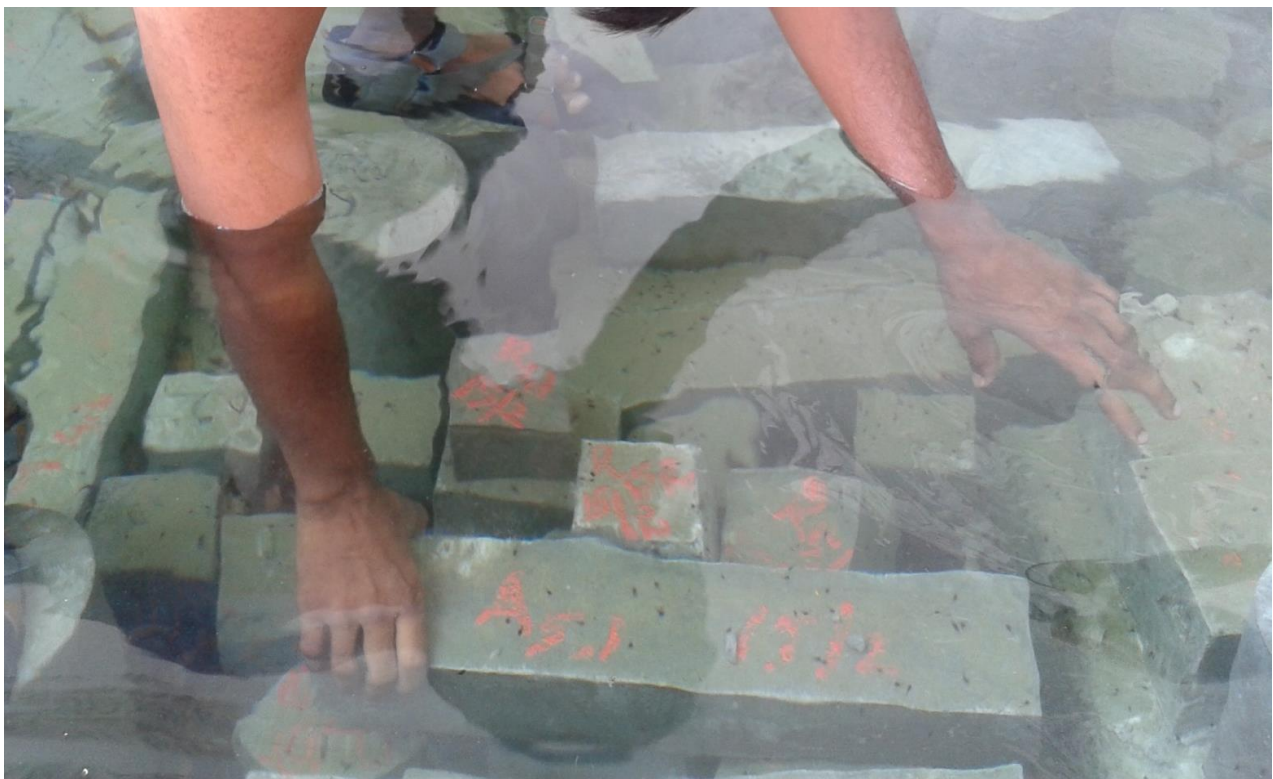
Fig.12: Placing dried samples in the curing tank
