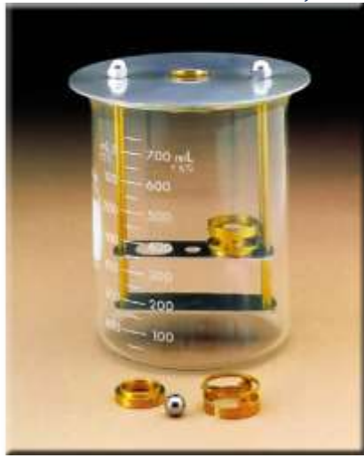
Figure 5.3.1: The component of the ring and ball test apparatus
