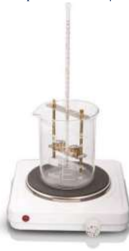
Figure 5.3.1: The component of the ring and ball test apparatus
