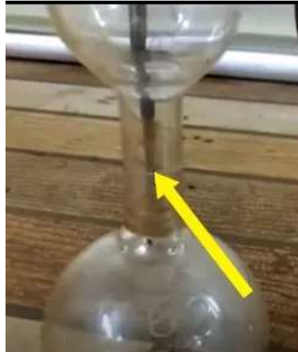
1. Fig 4.5a: Sample in viscometer
