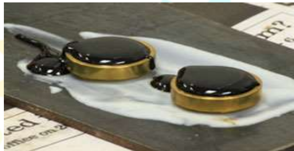
Figure 5.3a: The rings which contain bitumen, on a surface coated with a mixer of glycerin and dextrin.
