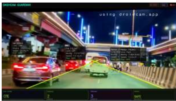
Fig: 3. System Output(night time):Real-time detection with HUD overlay.
