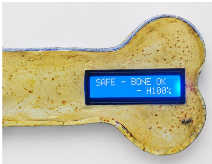
fig. 2. lcd display output showing the normal "safe" condition of the scaffold.
