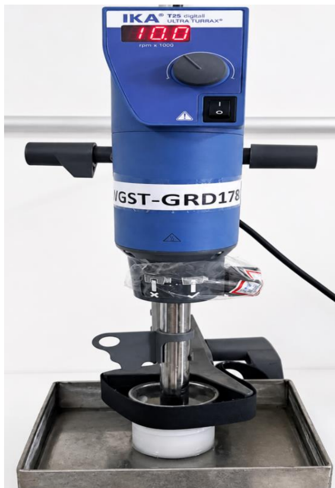
Fig. 1: Experimental setup for K-SLN preparation by high-speed homogenization.
