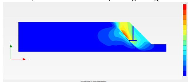
Figure 6 Deformation with a retaining wall
