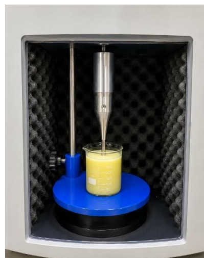
Figure 2: Probe sonication of the SLNs
