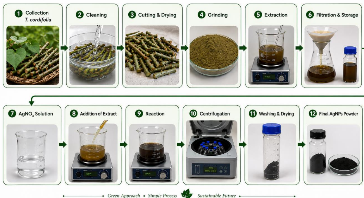
Figure 2: Schematic illustration of the green synthesis of Ag nanoparticles using T. cordifolia extract, showing the preparation of plant extract, synthesis process.
