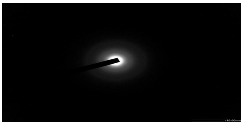
Figure 8: SAED pattern of T. Cordifolia -mediated Agnps indicating their crystalline structure.
