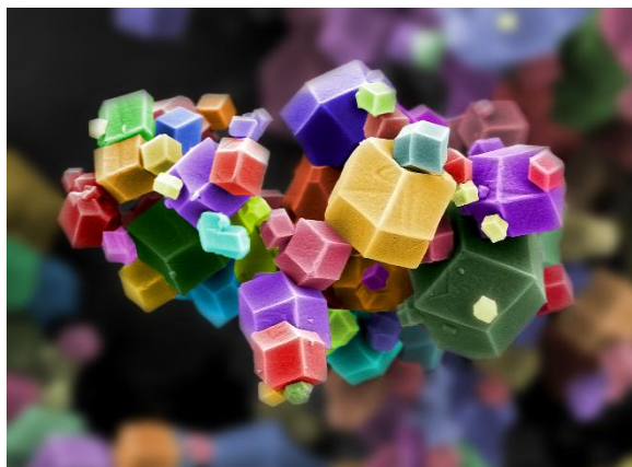
Figure 4. Representative high-resolution scanning electron microscopy image of metal-organic framework (MOF) polycrystals illustrating the micro/nanostructured morphology of MOF-based materials. Such porous architectures can provide large accessible surface areas and active sites for electrochemical sensing.
