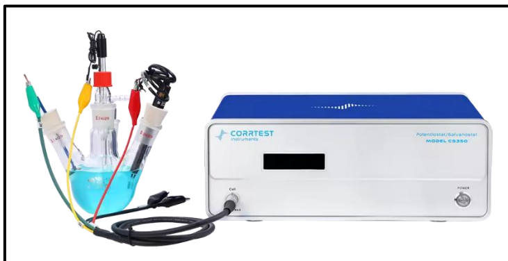
Figure 6. Representative potentiostat used for electrochemical measurements. Miniaturization of potentiostats is an important step toward portable and point-of-use electrochemical analysis of food constituents.
