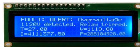
Figure1: output when overload detected
