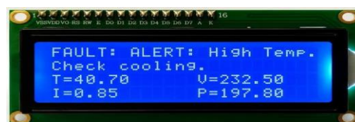
Figure3: output when over temperature detected
