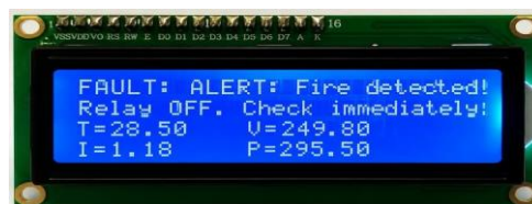
Figure. 2. Output when fire detected
