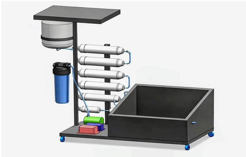
Figure 3.3. 2D & 3D CAD Model of the Proposed Hybrid Desalination System
