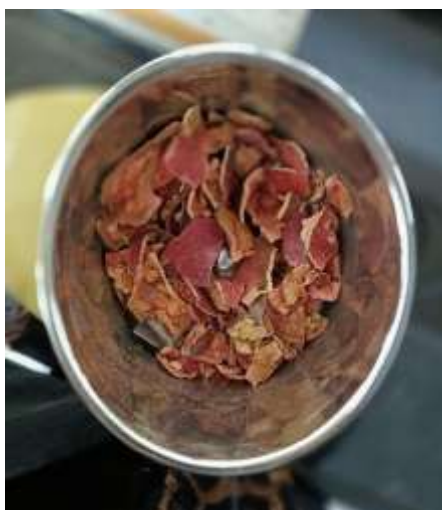
fig. 3: peel fragments undergoing particle size reduction in a mixer grinder
