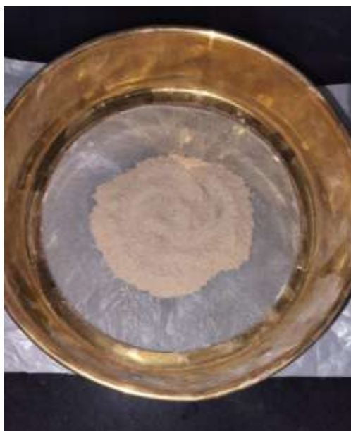
fig. 6: sieving of the powdered ingredient blend
