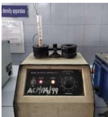
fig. 9: bulk and tapped density apparatus
