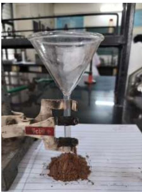
fig. 14: angle of repose determination by the fixed funnel method
