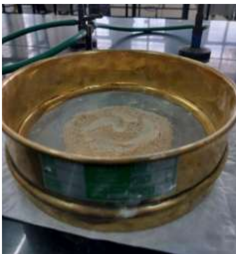
fig. 8: sieve analysis set-up used for particle size determination
