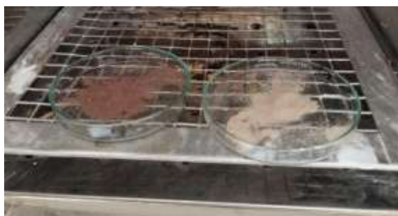
fig. 10: petri dishes in the hot air oven during loss-on-drying determination
