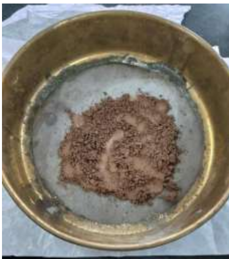
fig. 13: sieve analysis of vicco vajradanti tooth powder
