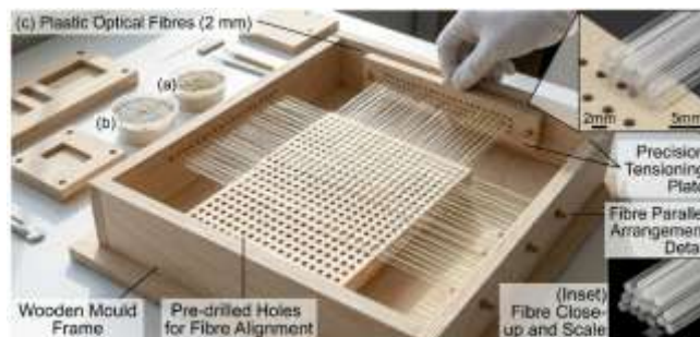
Fig. 3. Wooden mould with pre-drilled holes showing optical fibre arrangement in parallel orientation prior to casting.
