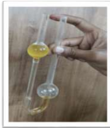
fig.no.12: determination of viscosity by using an ostwald viscometer.
