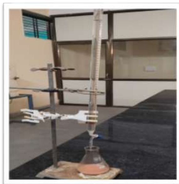
fig no.11: determination of acid value as a result pink colour convert in to pastel pink colour when titrate with 0.1n koh
