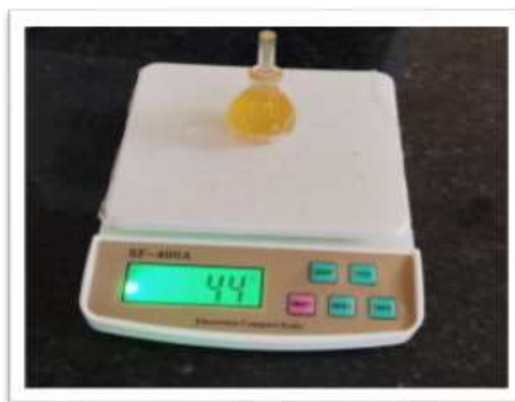
fig no.09: determine the specific gravity using density bottle.
