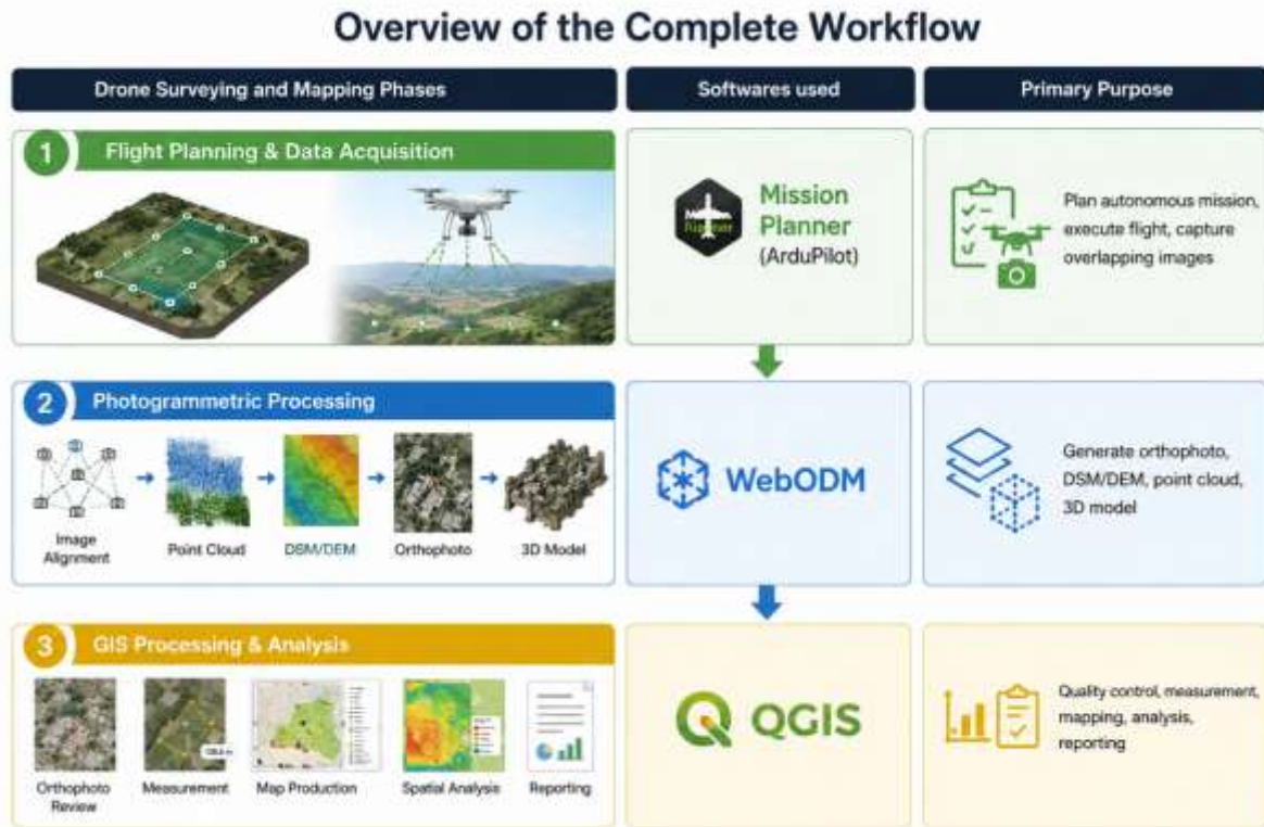
Fig.no 2: Drone Surveying and Mapping Phases (Software Approach)
