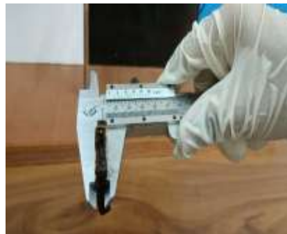
Fig no 11: Measurement of lozenge thickness using a Vernier caliper.
