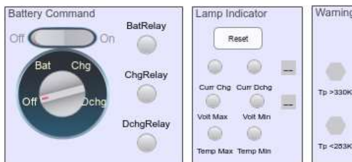
fig. 10. BMS Dashboard panel: Battery Command rotary switch, relay status LEDs (BatRelay, ChgRelay, DchgRelay), Lamp Indicator panel with six fault lamps and Reset button, and Warning hexagons for high/low temperature alerts
