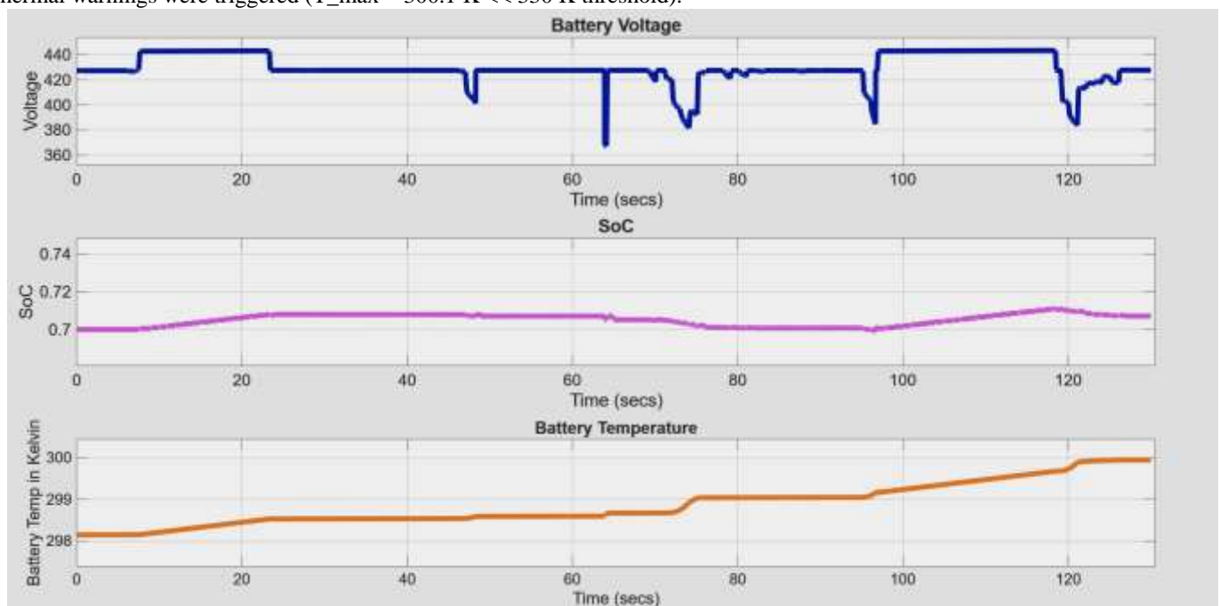
fig. 12. Simulation results — Battery state variables over 130 seconds: (top) pack terminal voltage ranging 362–441 V; (middle) AEKF-estimated SoC in the band 0.698–0.723; (bottom) battery temperature rising monotonically from 298.2 K to 300.1 K, well within both thermal warning thresholds.
