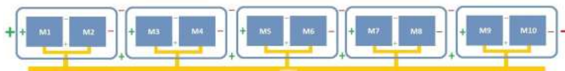
Fig. 2. Battery pack architecture showing ten series-connected module assemblies (M1–M10), each module containing two parallel cells, all sharing a common thermal bus for coolant-coupled thermal management.
