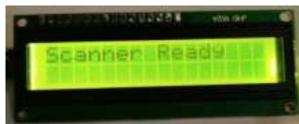
Fig.4(a) LCD module displaying system status message "Scanner Ready" after successful initialization
