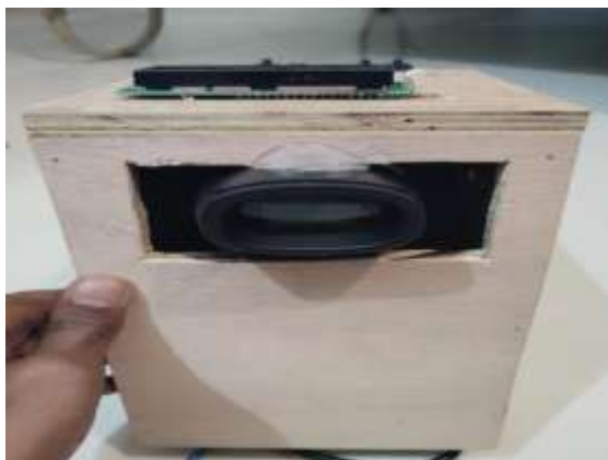
Fig 4(d) Barcode scanner mounted in the proposed system
