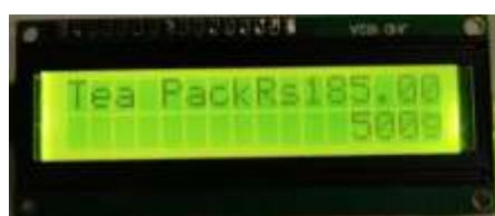
Fig.4(c) LCD displaying product name, price, and updated bill amount after barcode scan
