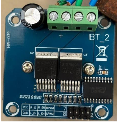
FIG.4: DC Motor Drivers.
