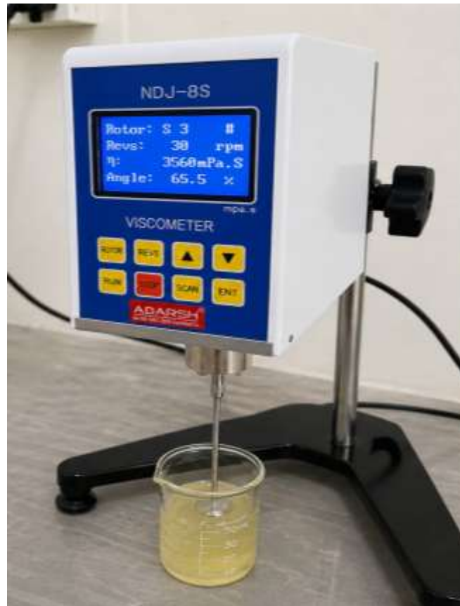
Figure 9: Determination of viscosity using viscometer
