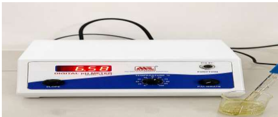
Figure 8: Determination Of Ph Using Ph Meter
