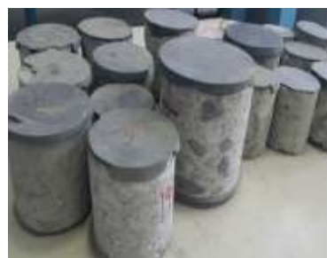
Figure 3.2: Collection of cement concrete core specimens for testing
