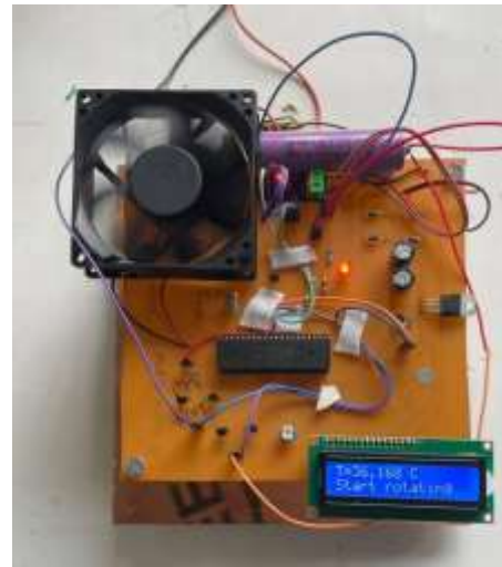
Fig. 5: T = 36.2^{\circ}\text{C} – fan on (start rotating)
