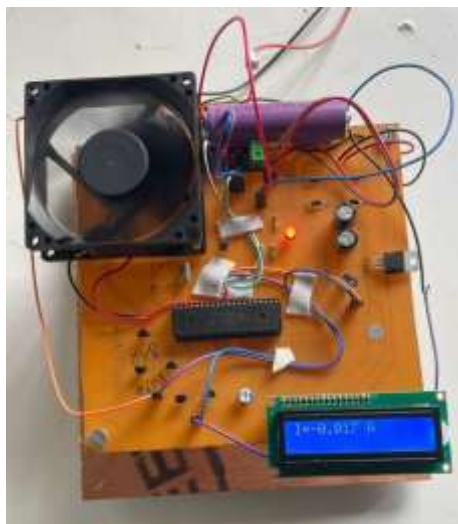
Fig. 3: Current measurement – I = -0.017\text{ A} (battery rest condition)
