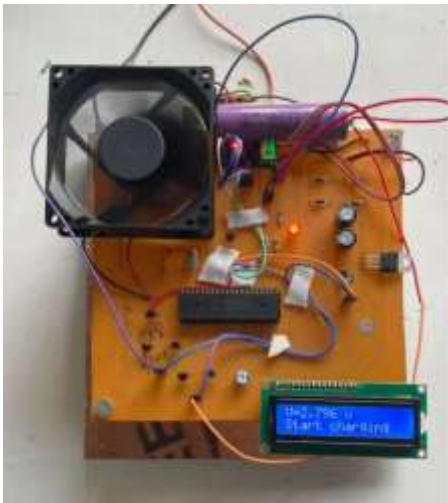
Fig. 1: V = 2.796\text{ V} – charging active
