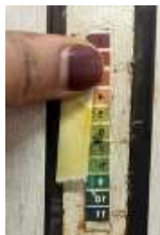
pH measured using pH paper and compared against the standard pH scale
