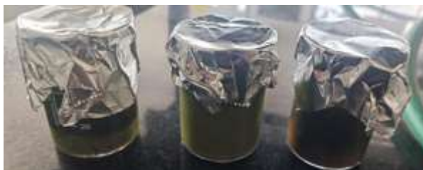
Guava, Neem, Tulsi leaves powder immersed in 90% ethanol & kept for maceration in a closed container
