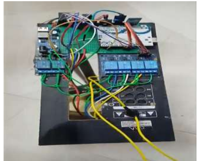
Fig. 8. Control box: Arduino UNO, relay module, HC-05 and DC-DC converter.
