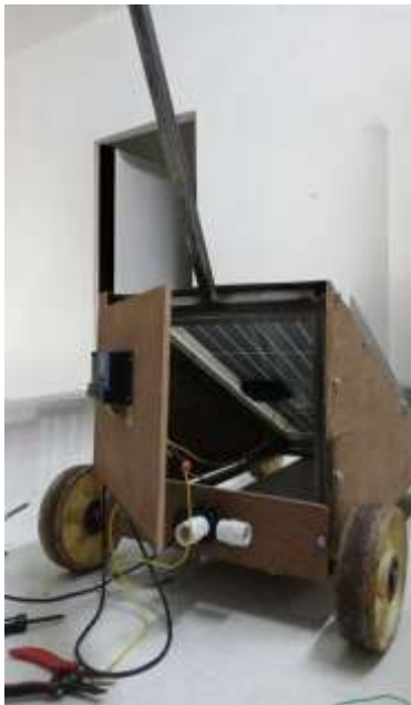
Fig. 7. Portable solar trolley with panel, battery and enclosure.
