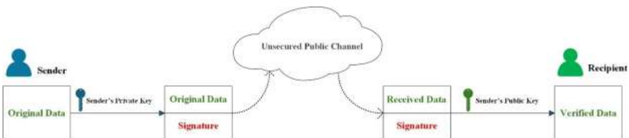
Fig. 2. digital signature operation using asymmetric-key cryptographic algorithms
