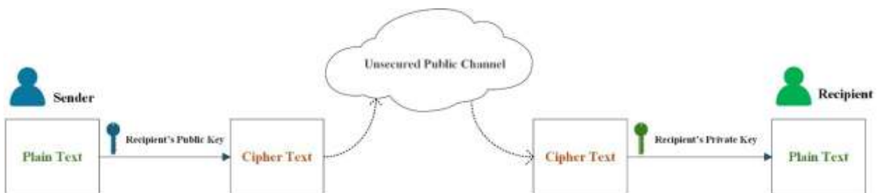
Fig. 1. encryption operation using asymmetric-key cryptographic algorithms
