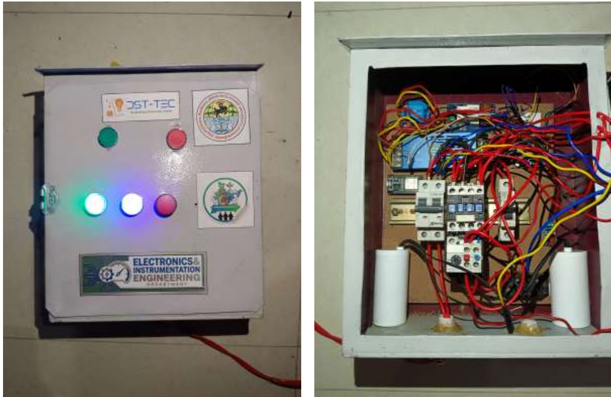
Figure 3: Front and inside views of the DOL starter unit.
