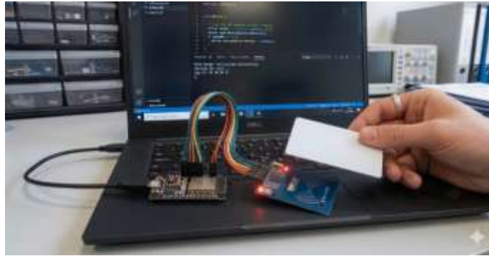
[Figure 2: Hardware Setup – ESP32 development board connected to MFRC522 RFID reader module with annotated pin connections (SPI bus: MOSI, MISO, SCK, SS, RST)]
