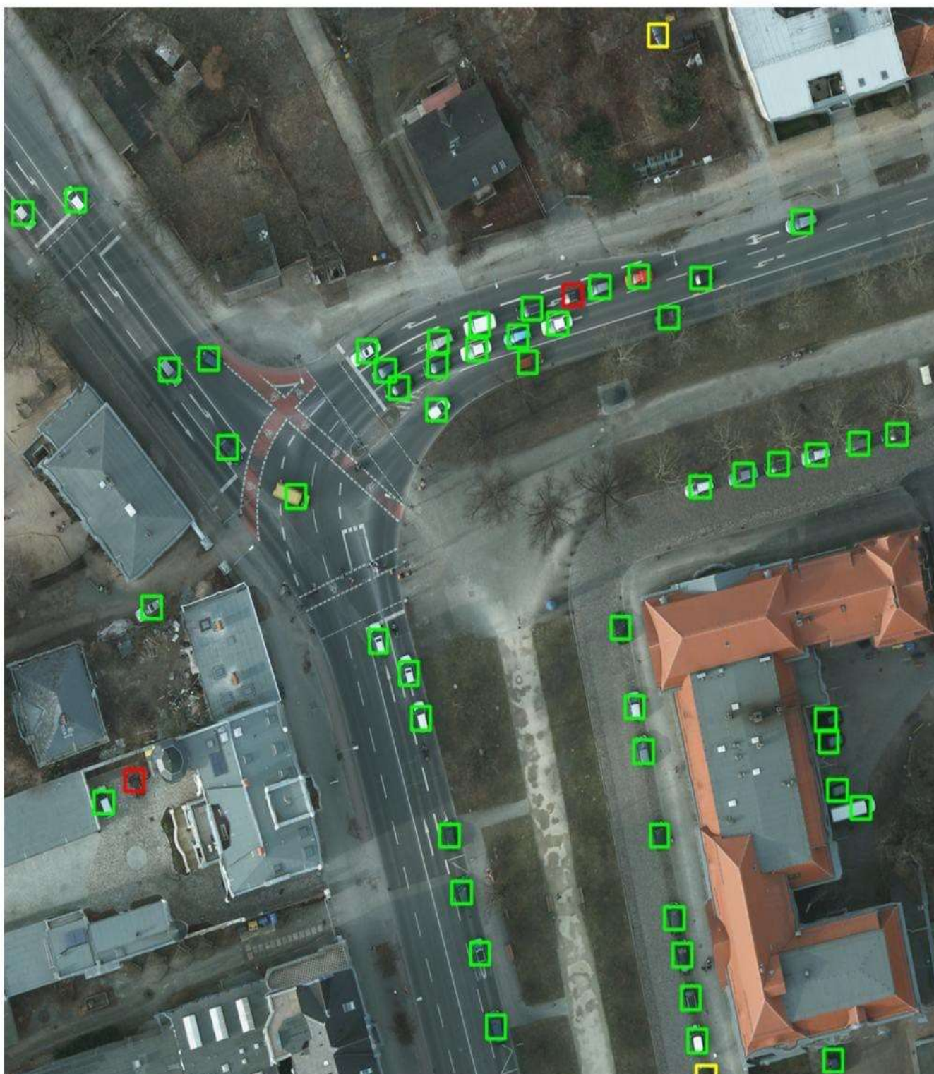
Fig. 5 — Drone Aerial View with Vehicle Detection (Green: Moving, Red: Stationary)
