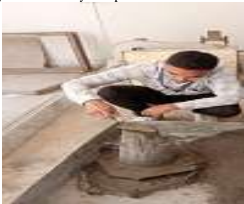
Figure No. 3.2 Workability Of Concrete By Slump Cone Method
