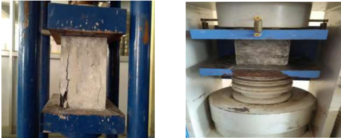
Figure No. 2.2 Compression test on Universal Testing Machine
