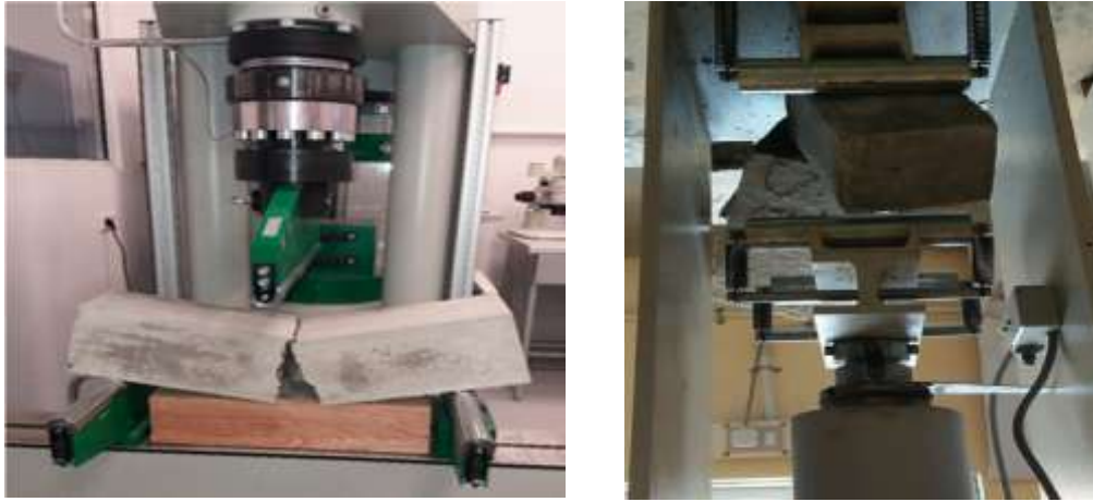
Figure No. 2.4 Flexural Strength test on flexure testing Machine
