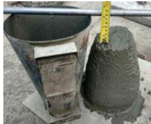
Figure No. 3.2 Workability Of Concrete By Slump Cone Method
