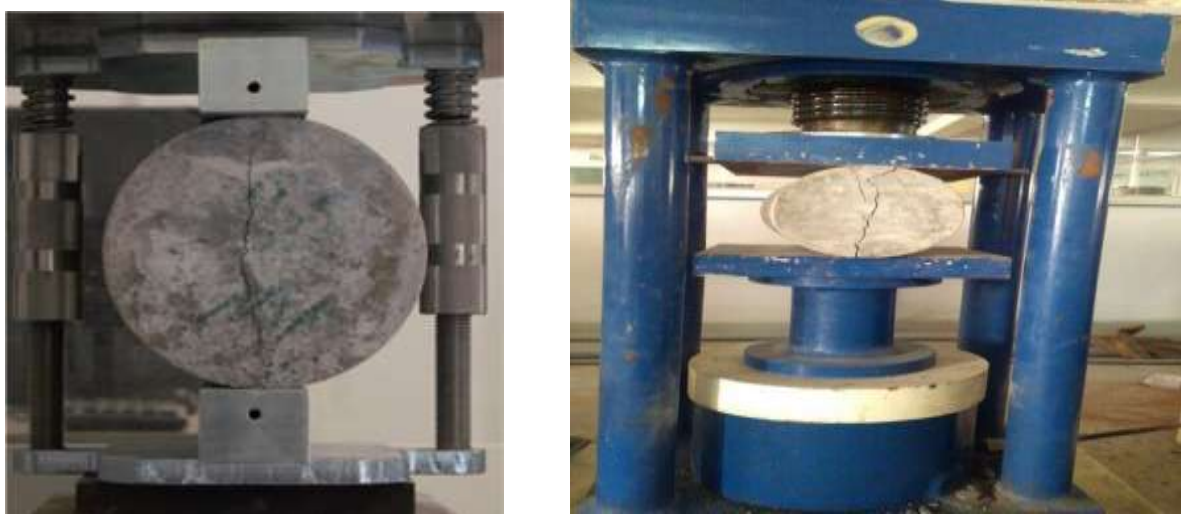
Figure No.2.3 Split tensile test on Universal testing Machine
