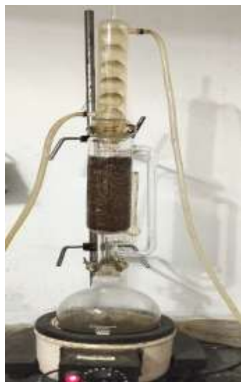
Soxhletation of Uraria picta with Methanol
