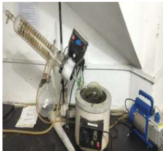
Rotary vacuum evaporator of Ethyl acetate
