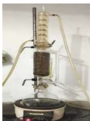
Soxhletation of Uraria picta with Ethyl acetate
