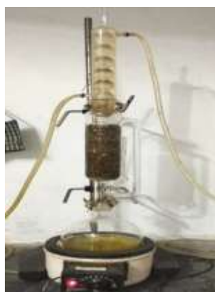
Soxhletation of Uraria picta with Petroleum Ether
