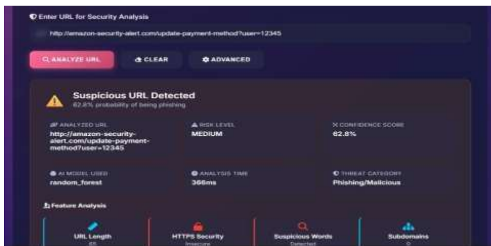
fig.4: It represents the analysed URL in the web page, and it categorizes the result by extracting the features of the URL
