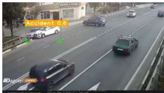
Fig. 2. Real time accident detection output using YOLOv8.
