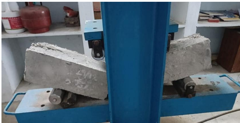
Fig.2. Experimental setup for flexural strength test
