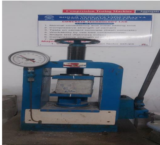
Fig.1. Experimental setup for compressive strength test
