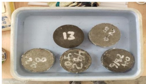
Fig. 15: Full immersion of cylindrical specimens for saturation test
