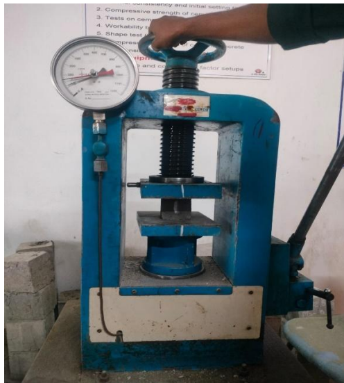
Fig. 7: Compressive strength test on trial 1 specimens
