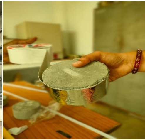
Fig. 13 : Sealing with aluminum tape
