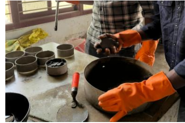
Fig. 5: Compaction of 3DPC cylinders
