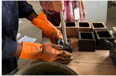
Fig. 4: Compaction of 3DPC cubes
