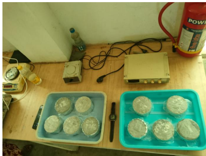
Fig. 14: Sorptivity test in progress — specimens placed in water tray
