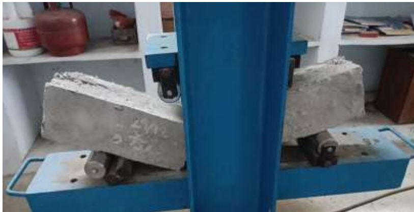
Fig. 2 Experimental setup for flexural strength test
