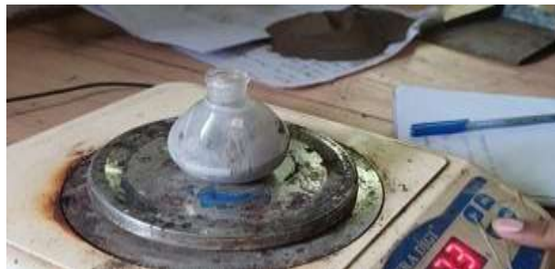
Figure 4: Specific gravity test setup(density bottle method).
