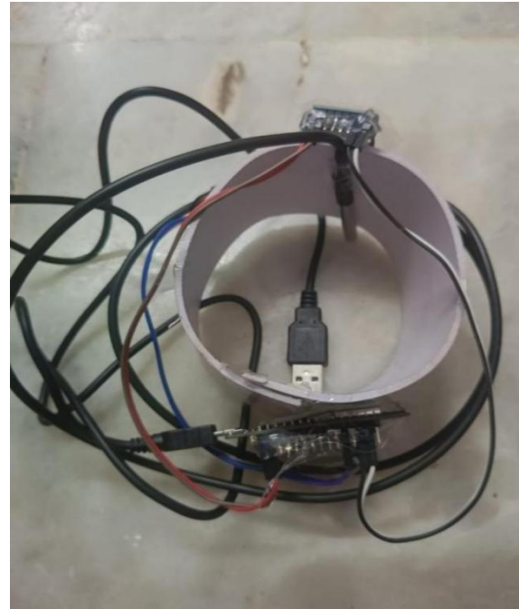
Fig.3 : Wrist Band which consists of Temperature and NIM Sensor
