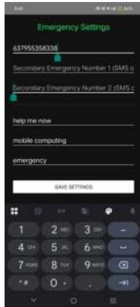
FIGURE 5: EMERGENCY SETTINGS INTERFACE OF ECHOGUARD, ALLOWING USERS TO CONFIGURE PRIMARY AND SECONDARY EMERGENCY CONTACT NUMBERS ALONG WITH PREDEFINED KEYWORDS FOR AUTOMATIC THREAT DETECTION AND ALERT ACTIVATION.
