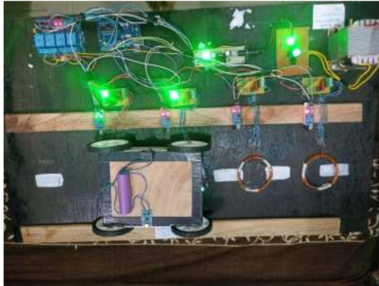
Fig. 3: Hardware prototype of smart EV on road charging system
