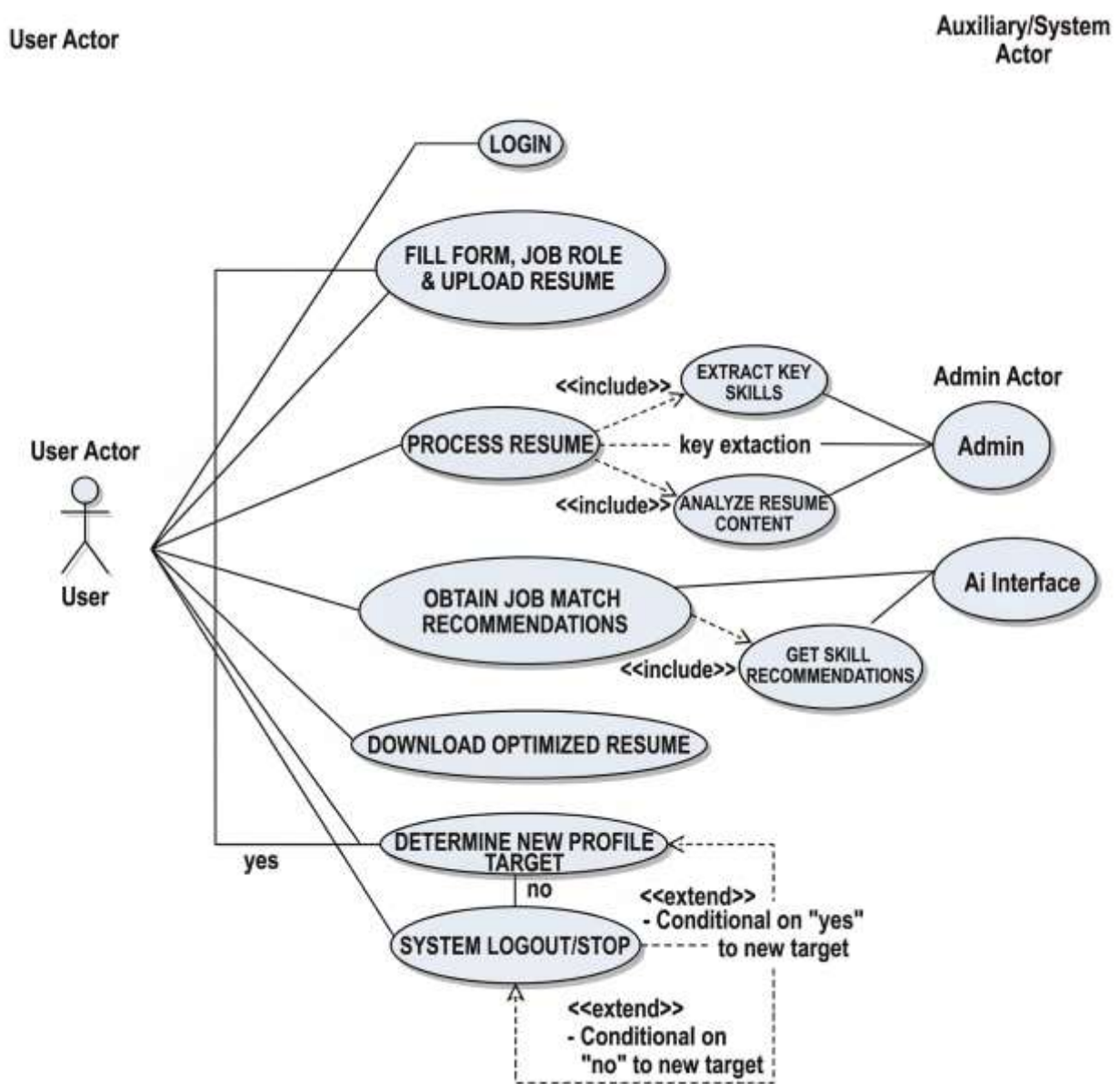
Fig. 2. Use case diagram of the proposed ResuMate system illustrating interactions between the user, admin, and AI interface during resume processing, job-role matching, and resume optimization.
