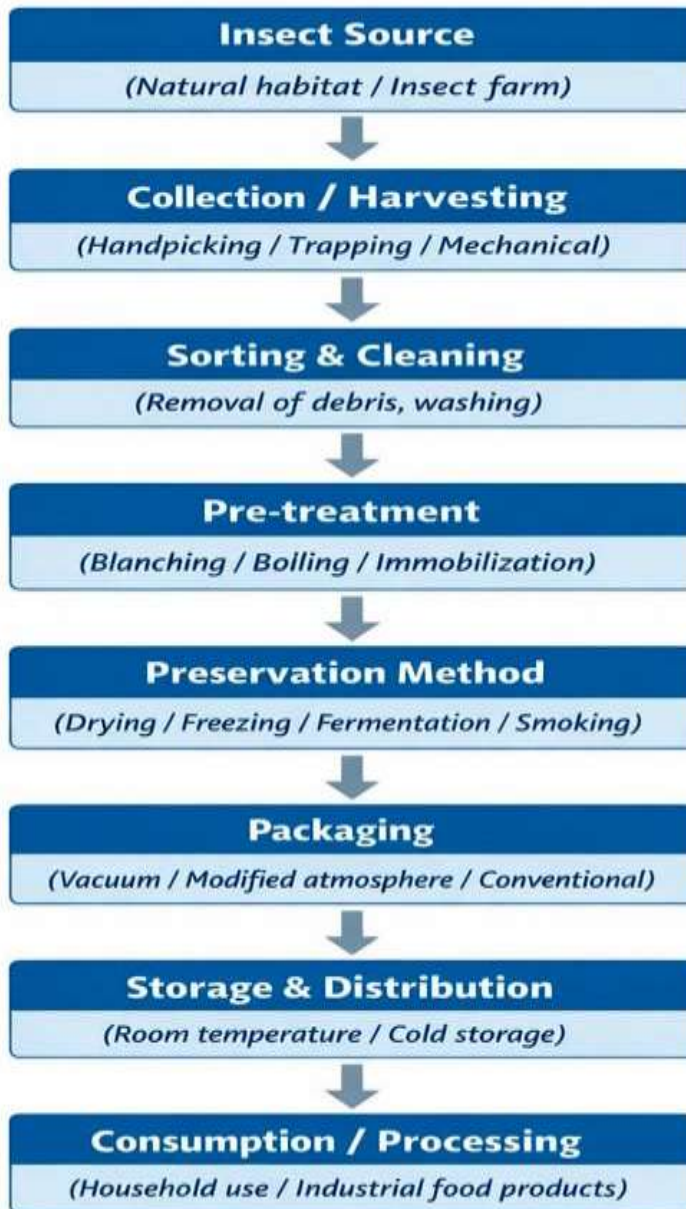
Figure 1 (recommended): Flow diagram of post-harvest handling and preservation pathways for edible insects.
