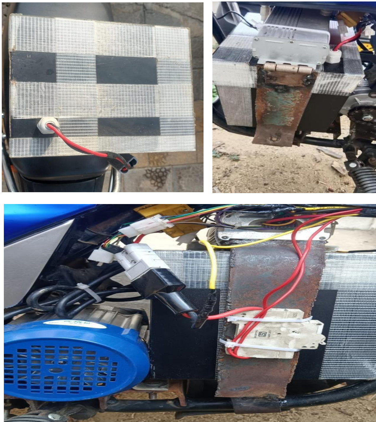
Figure 2: Battery Management System for Electric Bike
