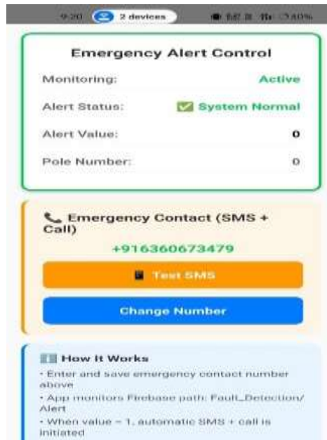
Fig.4. Emergency Alert Control API
