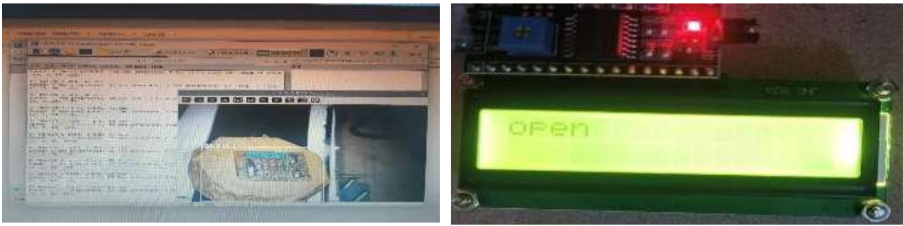
Fig. 6(c): Open-circuit defect
