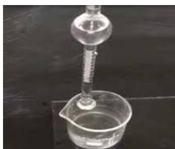
Determination of Surface tension using Stalagmometer
