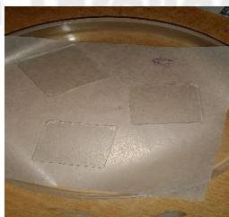
Figure 7. The image shows three glass substrates placed on a lining sheet inside a Petri dish after the completion of the coating and drying process. Each substrate exhibits uniform transparency, indicating that the \text{SiO}_2\text{--PDMS--wax} -based coating forms a continuous film without noticeable haze, cracking, or particulate agglomeration. The optical clarity demonstrates that the hierarchical \text{SiO}_2 nanoparticle layer remains
