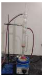
Figure 6.2: Extraction of plant material by soxhlet extraction
