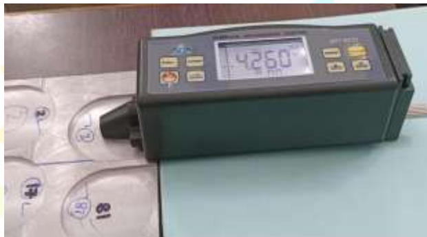
Fig. 4: Measurement of surface roughness using Talysurf tester
